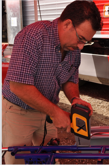
↑ Steel identification with an XRF analyser ↑
