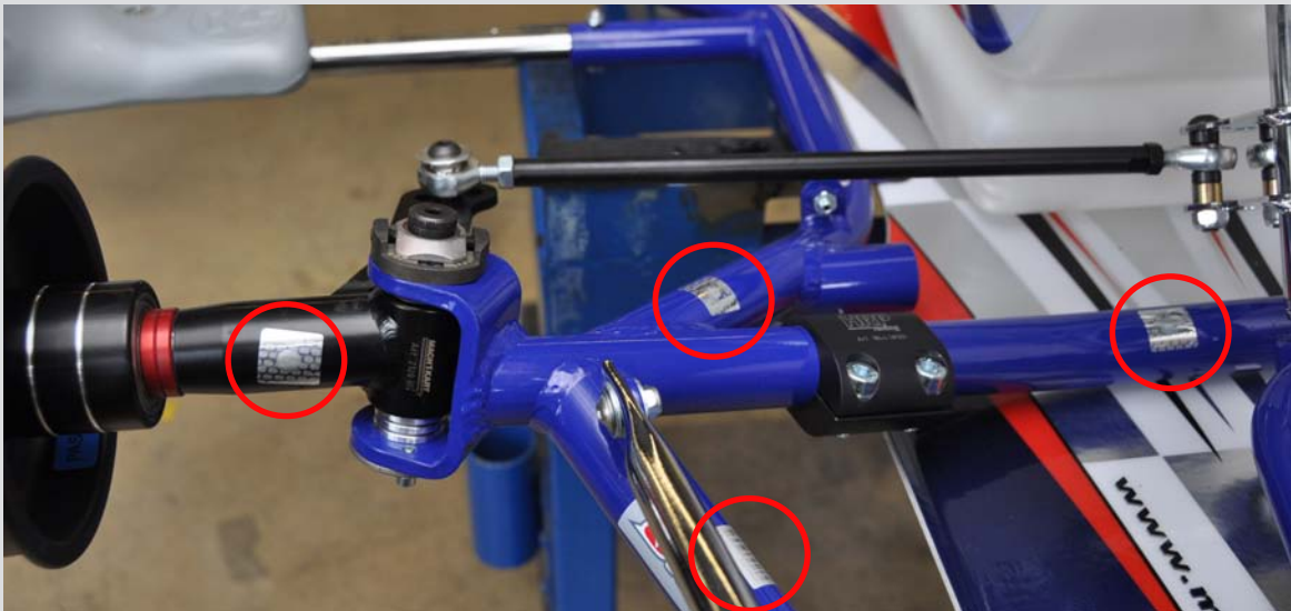
↑ Chassis and accessories marking (above: frame, stabilizer and spindle; below: rear axles) ↓
